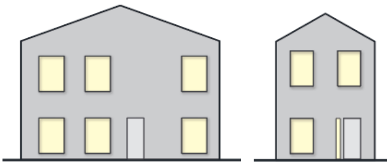
Figure 2.9.1 Diagram of 20% of street facing façade in glazing, for both narrow and wide sites
