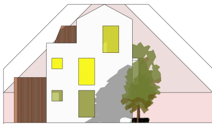
Figure 2.3.2 Street elevation of with side entry garage (this indicative example with 11m height and 5m+45° recession plane for front 2/3 of site and 2.8m+45° plane for rear 1/3)
