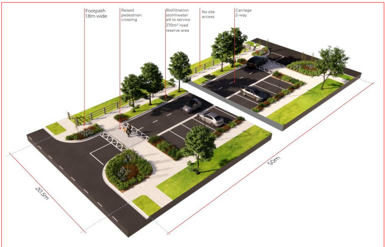
Figure 4-10: Indicative 20.5m Wide Cross Section Adjacent to Proposed Reserve (Road Type D)
