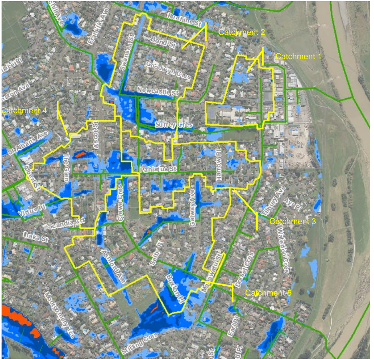
Figure 18: TUFLOW maximum ponding depths for 10% AEP (1 in 10-year) rainfall event with proposed catchment diversions
