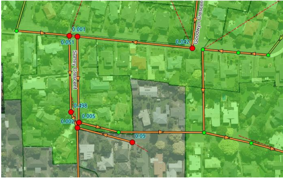
Figure 7: Zoom in of results for pre-development (existing land use) 10% AEP (Historical rainfall) event. [Surcharged pipes are shown in orange and red circles indicate spilling manholes. Spill volumes are shown in ML (1000 m³)]
